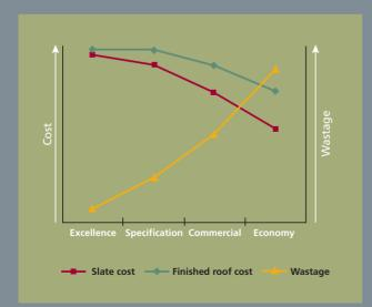
Note: all natural slates must be sorted prior to installation. When deciding on the most appropriate slate we recommend that you consider all of the costs associated. These include wastage rates, grading, sorting and trimming required with the lesser quality slates along with transportation costs needed for distribution.
